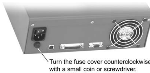
Figure 12: Replacing the fuse
